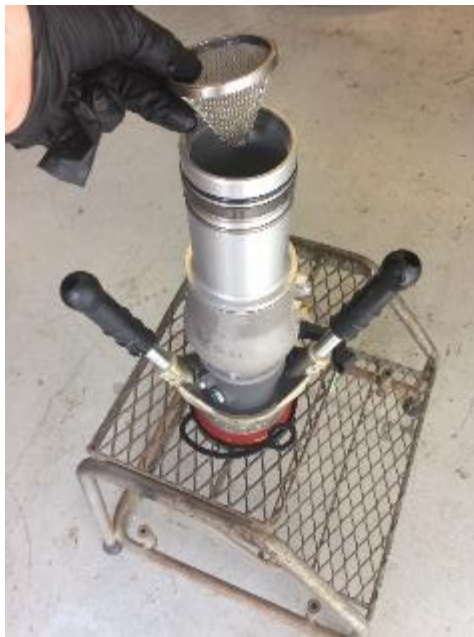
Left: Re-installation of the hose-end strainer into the hose end nozzle. Right: Clean hose-end strainer reinstalled with retainer ring in place.
