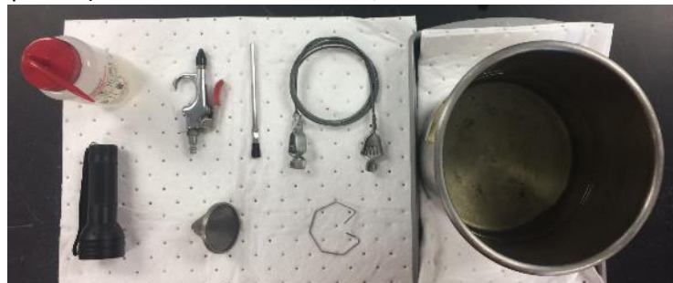
Equipment for hose-end strainer cleaning procedure.
