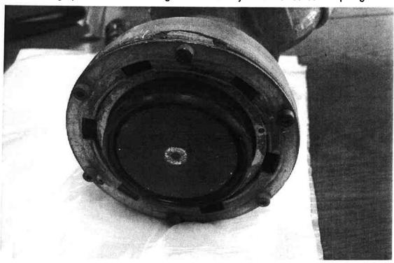
An investigation has indicated that the failures may be related to a manufacturing defect and a Service Bulletin has now been prepared by Carter and is available on <a href="https://www.argo-tech.com">www.argo-tech.com</a>. This Service Bulletin, SB200061005 dated July 11 2005, recommends that 64200 nozzles with serial numbers in the range 831 to 1088 be removed from service for inspection.
